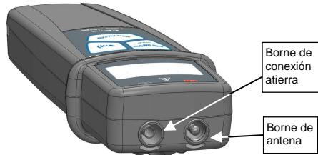
**2.3. Cara trasera (VX0003 y VX0100)**
