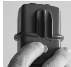
Hold the electric field tester keeping one of your fingers in direct contact with the correct area of the rear face of the appliance.
