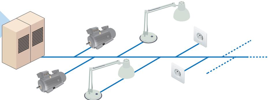
First, the technician takes measurements on the power supply for the lighting. He measures the harmonics on the voltage and current, as well as the transients. The results show that there are no transients and that the level of harmonics present is satisfactory.
