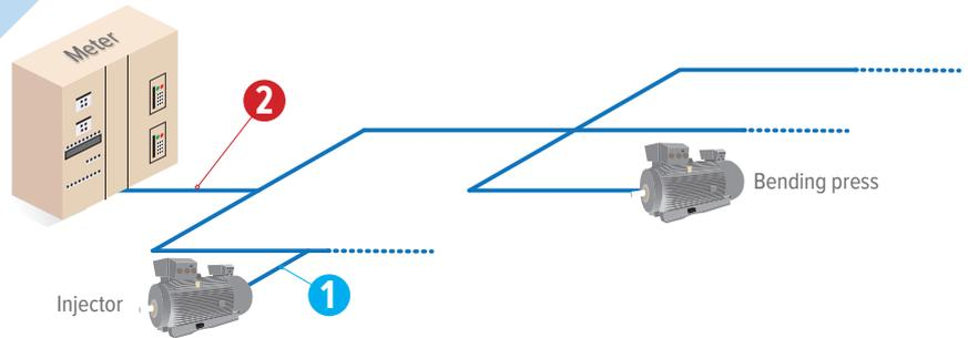
1 The instantaneous no-load voltages are OK. The Qualistar+ is then set up to record over several days. Analysis of the recording shows that voltage surges are occurring. These surges happen regularly on all three phases. This quickly calls into question the electricity supply, so monitoring is immediately resumed just downstream of the meter.
