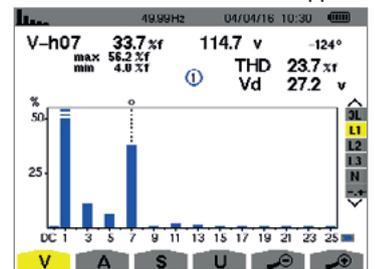
**Solution** : set up an anti-harmonic filter sized for the distorting current causing the fault.
