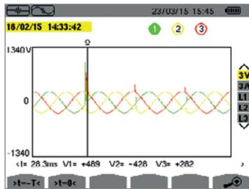
2 The new recording shows the presence of inrush currents and, above all, voltage spikes: each transient corresponds to a peak in the current. Only an old bending press is used in this workshop to manufacture the metal frames for boats. Suggested initially by the workshop technicians present, this line of enquiry was abandoned prematurely because the interruptions were not systematic when the bending press was in operation.
