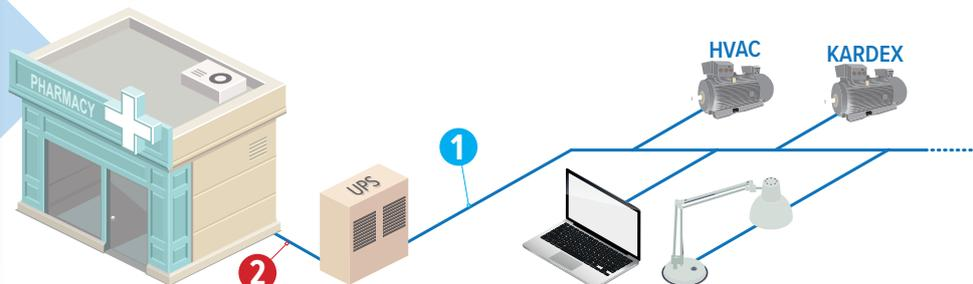
The first series of measurements 1, a trend recording, is performed on the output from the UPS. All the characteristics of the energy supplied are recorded and no anomalies are detected. The same characteristics are then measured upstream of the UPS 2. This time, the recording clearly shows a significant rise (several tens of Volts) in the Neutral/Earth voltage. The technician has noticed that these peak values occur when the street light comes on! In winter, the lights come on earlier!
