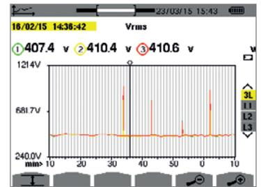
**Solution** : set up a corrective system on the electrical feeder of the bending press.
