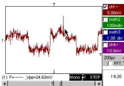
At first, after using the Autoset function or basic manual calibration, the signal form can be seen, but the trigger does not function correctly.
