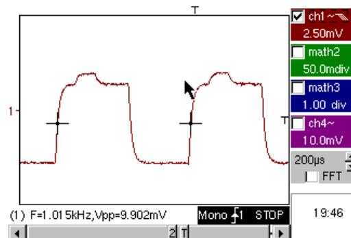
c) Use of averaging or curve smoothing (Horizontal menu) enables elimination of random noise on the visualisation (signal step serving as a trigger) and measurement of very weak levels after a vertical zoom.
