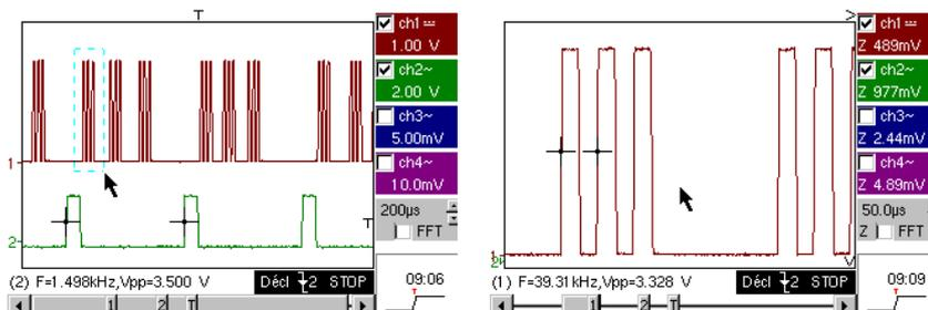
Using a timebase of 200 μs/div, graphically select the first group of 3 pulses and release to obtain the result.
