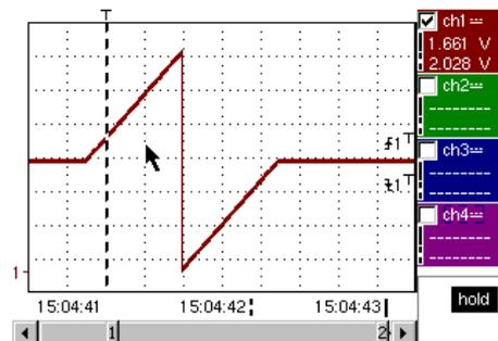
c) Using the "File Capture" option in the "Trigger" menu, we can detect and capture a whole sequence of faults and the instrument automatically stores the acquisitions in its memory (up to 510). In the following example we shall see how to sort and visualise them for analysis.
