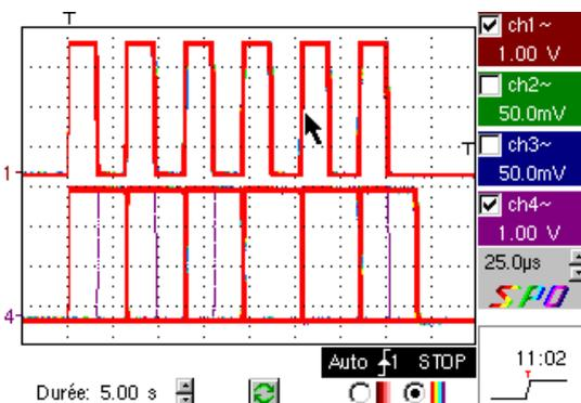
The proposed signal represents a communication bus with an "8-bit data" signal and a "clock" signal.
