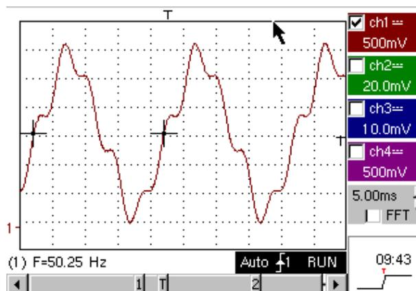
On electrical power distribution networks we regularly seek to observe possible harmonic distortion phenomena, which often cause problems for the global operation of the installation and the instruments connected.
