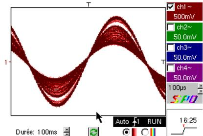
Due to its extremely high acquisition rate compared to a conventional Digital Oscilloscope (up to 50,000 per second instead of around 10 per second) and to its intelligent display algorithm, the SPO Oscilloscope enables visualisation of rapidly varying signals or complex composite signals, as possible on an analogue Oscilloscope.
