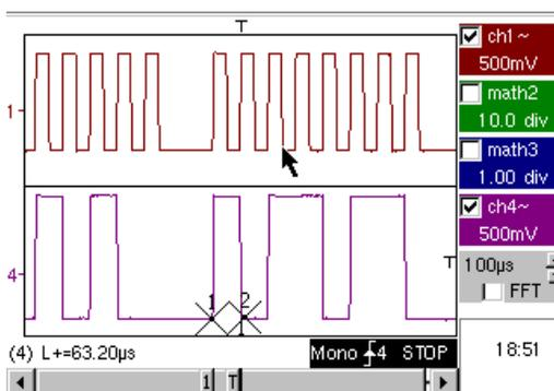
In normal "Oscilloscope" display mode, select to trigger on the AUX signal pulse width ("Trigger" menu - "Pulse" tab).
