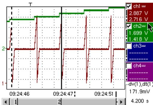
The two vertical cursors, one a dashed line and the other a full line, enable us to take 2 amplitude measurements for each channel simultaneously.
