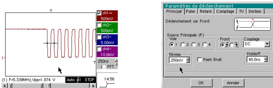
Then set up a pulse-width trigger as indicated below, and increase the timebase speed in order to allow detailed analysis of the fault on the digital frame.
