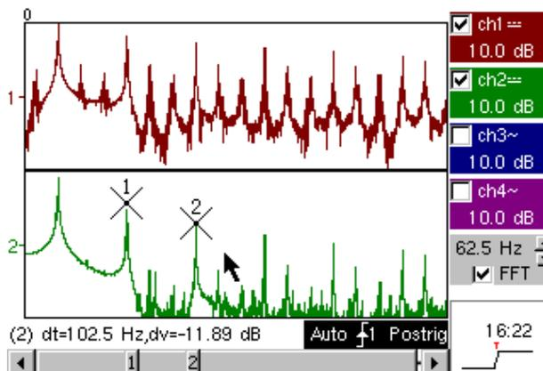
In linear mode the amplitude scale is expressed in volts, in logarithmic mode in dB, offering a greater analysis dynamic (49dB for a traditional 8-bit Oscilloscope, 60dB for the OX6000 and 79dB for Scopix and its 12-bit conversion).
