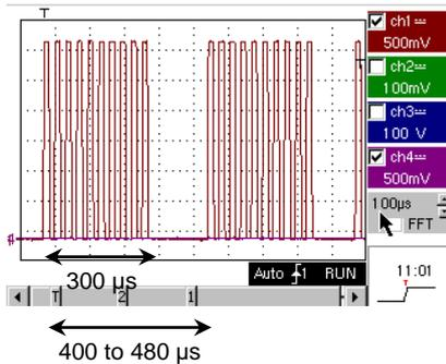
The correct selection of the "Hold-Off" parameter in the "Principal" tab of the Trigger menu will enable you to systematically trigger on the first pulse in the train.
