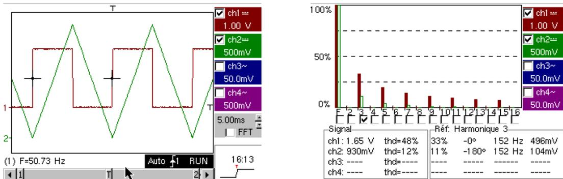
This instructive example uses two highly characteristic signals, a square and a triangle, and through analysis of harmonics enables verification of the theory of decomposition of fundamental signals.
