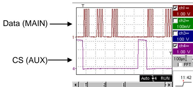
b) We will now demonstrate the interest of complex triggers (2 sources) with the “count” or “delay” options. The example provided will enable the synchronisation of an auxiliary signal, the Chip Select, with triggering on the desired pulse in the data frame. Additionally, this mode will enable us to always trigger on the same pulse even if it does not arrive at an identical interval after the chip select (pulses 4 to 9).
