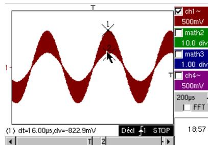
On the OX 6000 and Scopix models the Envelope and Cumulate (OX 6000-II & SCOPIX) modes enable rough visualisation of the signal (max Vpp, modulation rate, frequency, etc.).
