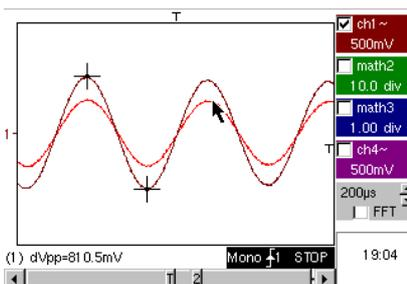
In the "Automatic Measurements" panel, a check box lets you display the difference between the current acquisition and the memorised reference (e.g. dVpp = difference in Vpp value).
