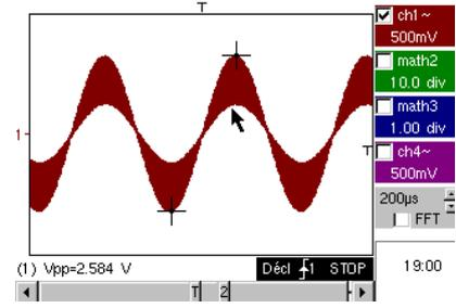
c) On our Oscilloscopes, it is possible to rapidly create a reference for comparison with a new acquisition (see test no. 3, final part).
