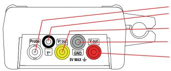
One BNC socket for the measuring probe.
