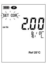
Press the SET key and set the TDS factor (f) to between 0.40 and 1.00 using the ▲ and ▼ keys. A sustained press on ▲ or ▼ scrolls through the values faster.
