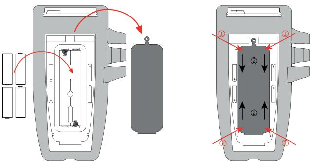
Put the battery compartment cover back in place; make sure that it is completely and correctly closed.
