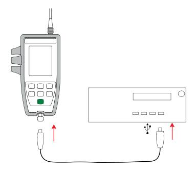
Once the Data Logger Transfer software has been installed, connect the instrument to the PC.
