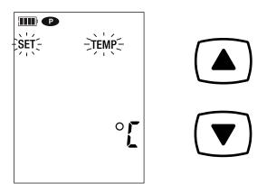
■ Press the **SET** key and use the ▲ and ▼ keys to set the temperature correction.
