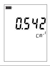
During the calibrations, the cell coefficient for a given cell must vary only a little. If you observe a large variation, it may be necessary to redo the calibration, check the condition of the standard solution (in particular the use-by date), or replace the cell.
