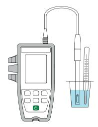
The instrument displays the conductivity measurement and the temperature measured, the reference temperature and the time. ATC = Automatic Temperature Compensation
