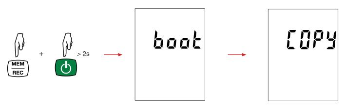
Release the keys and the instrument displays **COPY**, indicating that it is ready to receive the new software.
