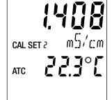
Confirm the set by pressing the CAL key. The instrument displays the measured conductivity and the temperature.
