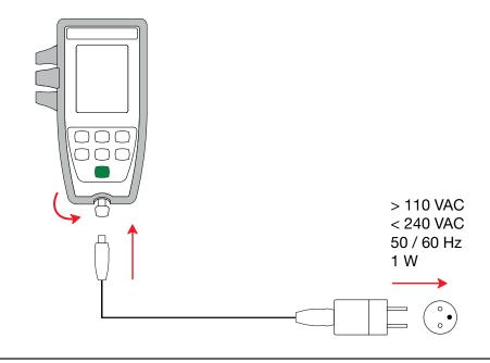
Connecting the external USB supply does not recharge the storage batteries.
