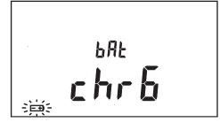
bAt on the small display and FULL in the main display means that charging is completed.
