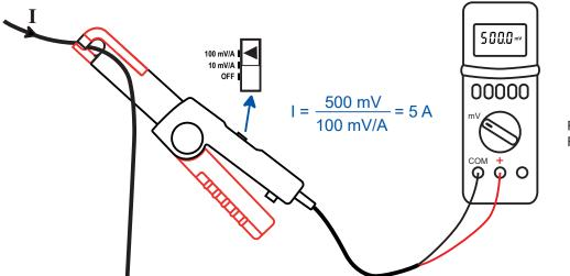
Rango 100 A 10 mV/A Rango 10 A 100 mV/A
