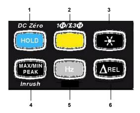
Figure 3: the keys of the keypad
