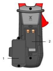
Figure 6: the battery compartment cover
