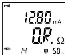
When the impedance measurement is >1200Ω, the instrument indicates **OR.**
