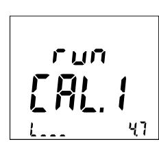
**Step 4/7.** The instrument performs the second part of the current measurement adjustment.
