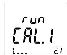
**Step 2/7.** The instrument performs the first part of the current measurement adjustment.
