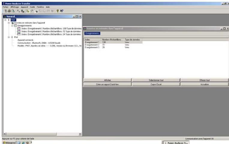
3.3 The data are recovered in PAT software. Display of the data in Text mode, in the format « date – time – MIN – AVG – MAX ».
