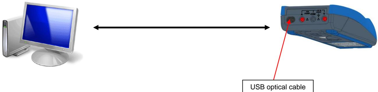
If your instrument has the Bluetooth option and your computer also has it, or a Bluetooth dongle, you can use the virtual com port created after connection to remotely program your instrument just as you would with a USB/optical cable
