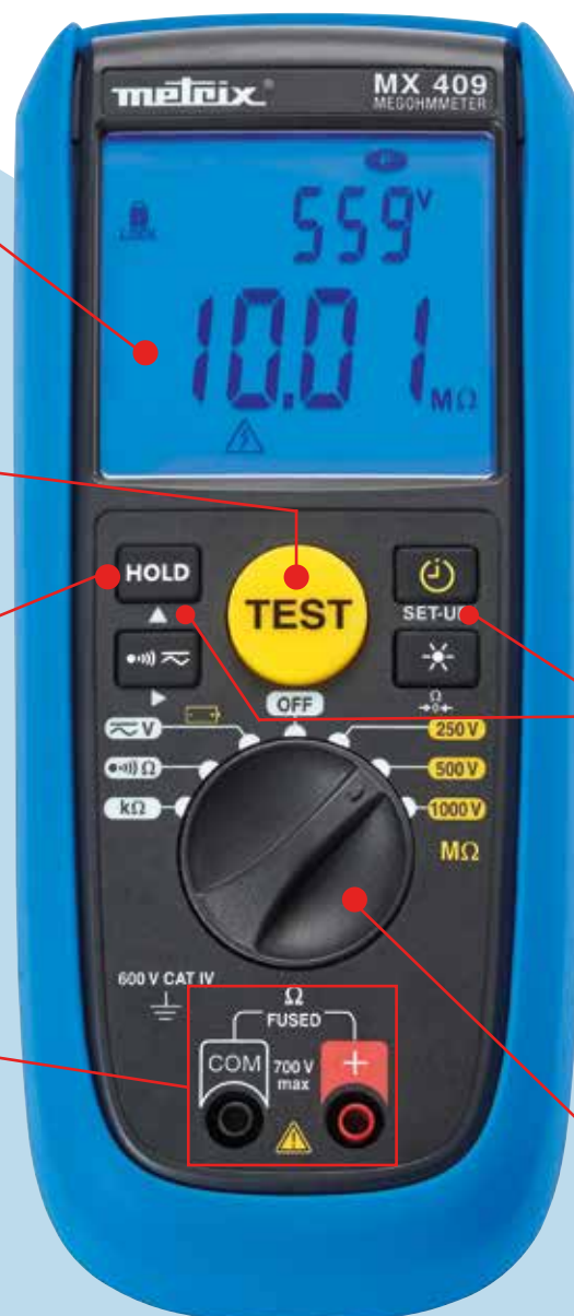
HOLD: automatic freezing of the display at the end of each measurement
