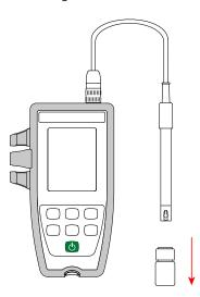
■ Rinse the electrode in de-ionized water, then dry it.
