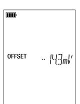
During the calibrations, the offset of a given electrode must not vary more than a little. If you observe a large variation, redo the calibration. If the problem persists, check the buffer solution (in particular the use-by dates) or replace the electrode.
