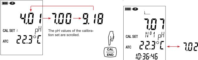
The instrument performs the pH measurement and indicates its progress.
