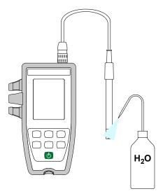
■ Pour each buffer solution (one, two, or three depending on the number of calibration points) into a beaker. The third buffer solution (NIST, pH 9.18) is an option.
