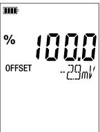
■ If you want to continue the calibration, withdraw the electrode from the solution, rinse it with de-ionized water, dry it, plunge it in the second buffer solution, and press the **CAL** key again.
