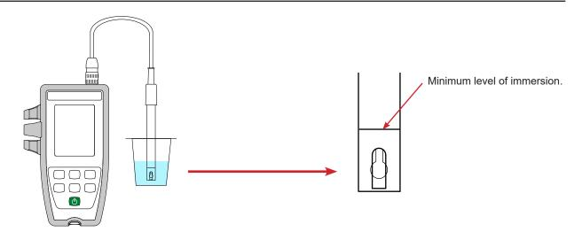
The electrode supplied with the instrument has an integrated temperature probe. There is therefore no need to measure the temperature of the solution.
