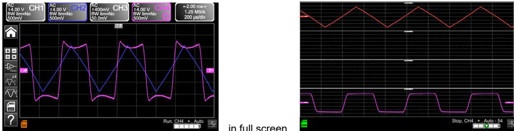
b) Select the XY mode with CH1 on X and CH4 on Y ; add 20 automatics measurements.
