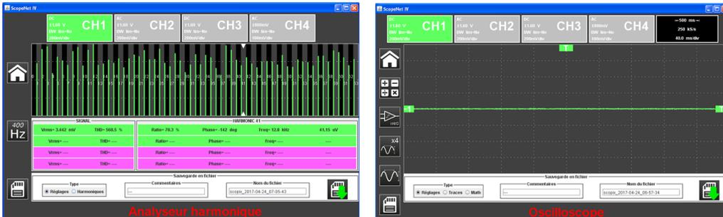
When you have obtained the IP address of the Scopix IV (DHCP or manual) using a browser, type 14.3.250.51/scopenet.html (for example) on your computer → this opens the screen shown opposite.
