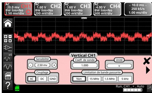
b) The use of the 1.5 MHz and 5 kHz analogue filters on the input will enable correct synchronisation and analysis of the signal free of any noise.
