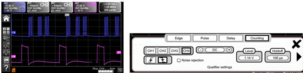
b) We will now demonstrate the interest of complex triggers (2 sources) with the «count» or «delay» options. The example provided will enable the synchronisation of an auxiliary signal, the Chip Select, with triggering on the desired pulse in the data frame. Additionally, this mode will enable us to always trigger on the same pulse even if it does not arrive at an identical interval after the chip select (pulses 4 to 9).
