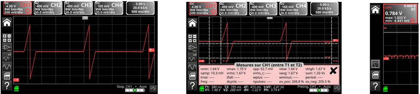
b) Select «logger» mode (Recorder) and calibrate 500 mV/div. fix duration of 10 000 s with resolution of 0.2 s on the on home screen: automatic recorder on files .rec.
