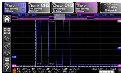
Using a time base of 200 μs/div., graphically select the first group of 3 pulses and release to obtain the result Zoom simultaneously with waveform..
