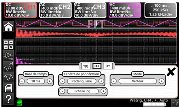
In linear mode, the amplitude scale is expressed in volts, in logarithmic mode in dB, offering a greater analysis dynamic (79 dB for SCOPIX IV and its 12 bits conversion).
