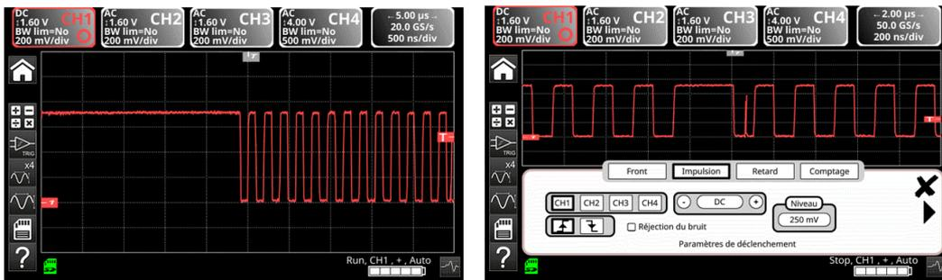
Then set up a pulse-width trigger as indicated below, and increase the time base speed in order to allow detailed analysis of the fault on the digital frame.
