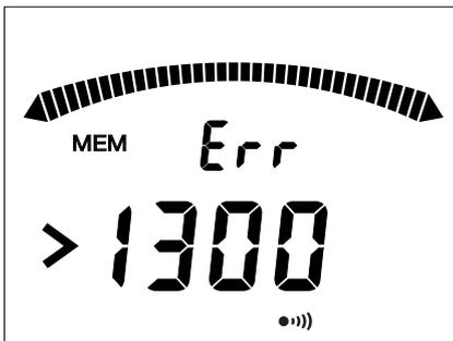
When the memory is full, it is no longer possible to record measurements and the instrument displays the screen shown opposite.
