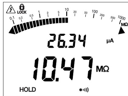
Then long-press the **MEM** key to store the measurement. The measurement is recorded in the first memory slot
