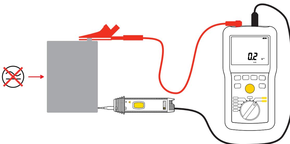
When the probe is connected, the
