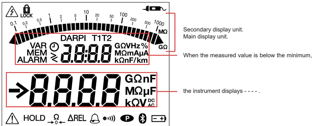
In voltage measurement, when the measurement exceeds the limit (either positive or negative), the instrument displays OL or -OL.
