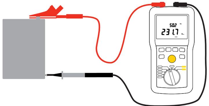
The instrument displays the voltage on the terminals. It detects whether the voltage is AC or DC and, if it is AC, the C.A 6532 also displays the frequency.
