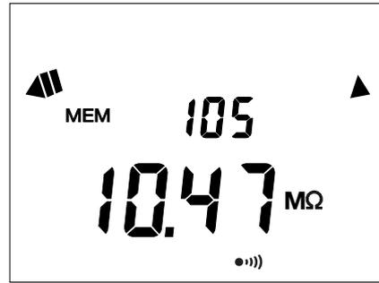
To see the other measurements, press the ▲ key. The record number is decremented and the corresponding measurement is displayed. To scroll rapidly through the recorded measurements, keep the ▲ key pressed.
