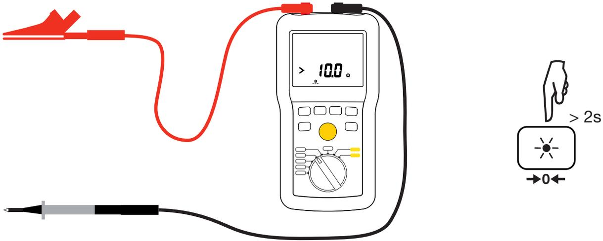
The display indicates the resistance of the leads and the  $\rightarrow \Omega \leftarrow$  symbol goes off.
