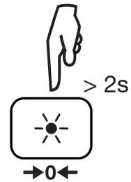
The display changes to zero and the →0← symbol is displayed. The resistance of the leads will be systematically subtracted from all continuity measurements. If the resistance of the leads is > 10 Ω, there is no compensation.
