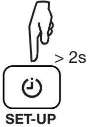
A long press on the SET-UP key is used to enter the configuration (set-up) function of the instrument.
