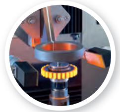
Example: Heating by induction for surface hardening of gears Photo Credit: EMAG eldec Hardening Systems
