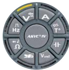
Digital keypad which lights up the active function, storage of configurations
