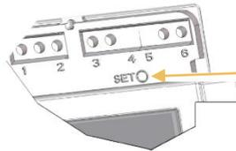
For preliminary setup, press the SET button for at least 4 sec
